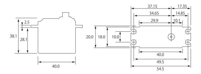
RATED VOLTAGEDC6.0V~7.4VOPERATING VOLTAGE DC4.0V~8.4V▲ CAUTION• No dry battery use
