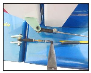
Crimp the brass tube with a crimping tool or pliers.
