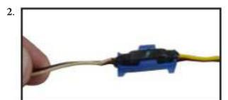
Fasten the pull string from the servo hole to the male plug of the servo extension.
