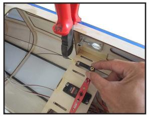
Cut off excess cable as shown.
