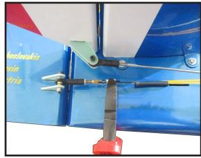
Cut off excess cable as shown.
