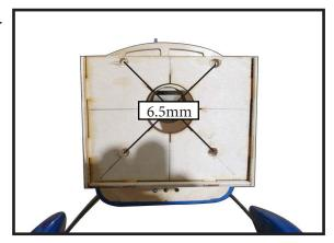
Attach the motor mount to the front of the electric motor box using four 6.5mm blind nut, four M5x25mm hex head bolts to secure the motor. Please see picture shown.
