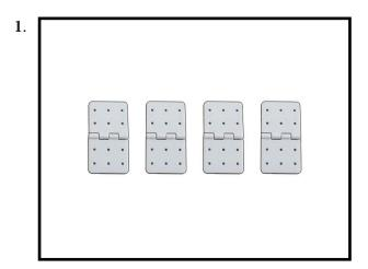
Prepare the aileron hinges by scuffing the area that will be inserted into the wing or flying surface with medium grit sand paper. Be careful not to remove too much material. Use isopropyl alchol, and a paper towel to remove any excess debris that remains on the hinges.
