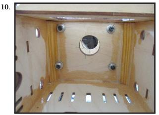
Attach the electric motor box to the firewall centered with the cross lines drawn on the electric motor box and firewall. Using M5x35mm to secure the motor box to the firewall. Please see pictures below.
