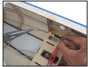
Crimp the brass swage tube with a crimping tool or pliers.
