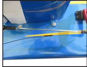
Thread cable through brass swage tube.
