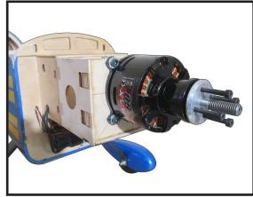
Attach the speed control to the side of the motor box using two-sided tape and tie wraps. Connect the appropriate leads from the speed control to the motor. Make sure the leads will not interfere with the operation of the motor. *17*.
