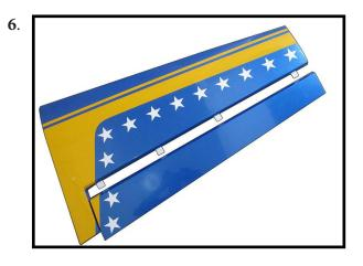
Press the aileron and wing together such that less than a 1/64" hinge line gap exists between the aileron and wing. The bevels should virtually touch. Use a paper towel and rubbing alcohol to wipe away any visible epoxy around the hinges.
