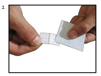
Mix a sufficient amount of 30-minute epoxy in a cup, and with a toothpick, smear epoxy in the hinge pockets of the wing panel and aileron. Slowly and carefully, insert each hinge into the wing panel. Partially remove and reinstall the hinge to ensure that you've completely coated it with glue. Clean up any excess epoxy with isopropyl alcohol, and tape the aileron in place to cure.
