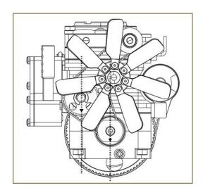
Diagram of Timing belt, please confirm that the marking points are consistent
