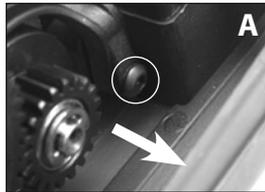
3. Disconnect the throttle return spring from the clutch guard.
