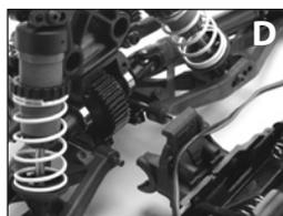
9. Remove the two 4x12 button-head screws from the rear shock tower and the two 3x15 button-head screws from the rear camber links (E) to separate the rear suspension system from the transmission.
