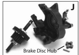
14. Remove the screw pin from the input gear and slide the input gear off of the shaft. (K)
