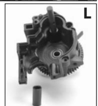
15. Remove the two-speed hub/gear assembly from the right half. (M) **Note:** The two-speed hub/gear assembly is not used with the single-speed conversion.
