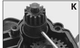
**Note:** Do not remove the plastic spacer located behind the input gear. The plastic spacer included in the single-speed kit is the *same* size as the two-speed plastic spacer. Only one spacer is used. The extra spacer can be saved for a spare. (L)
