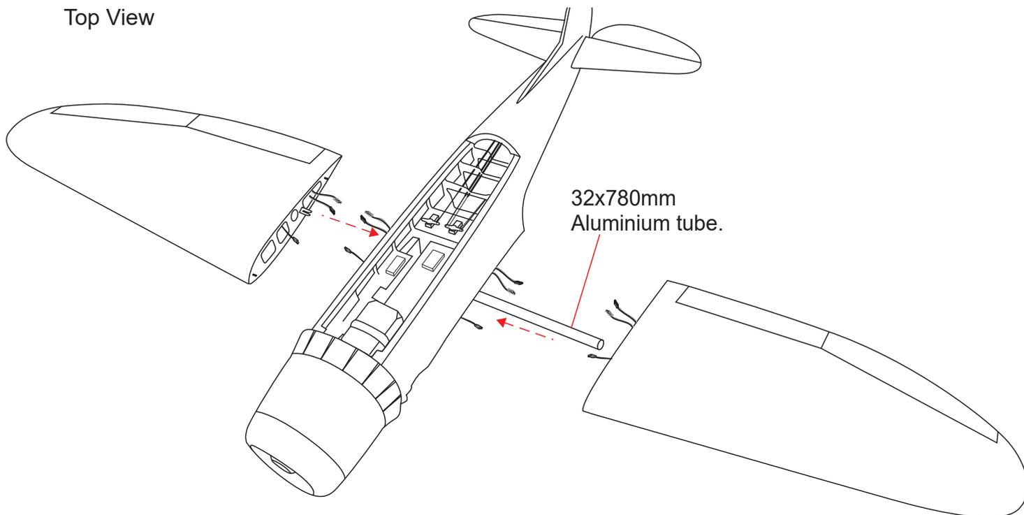
Main wing must be inserted and attached completely before fixing with screw.
