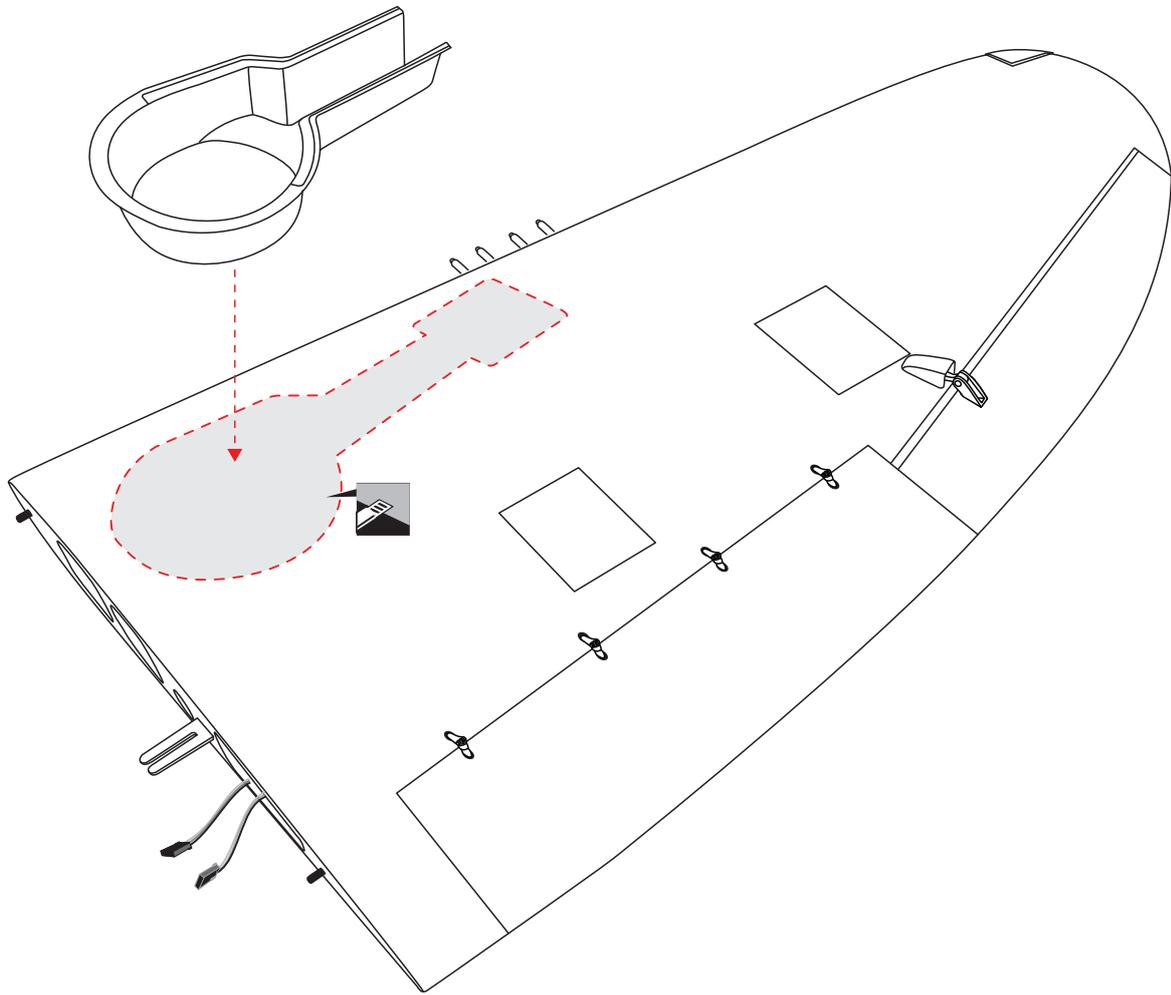
Using a modeling knife, carefully remove the firm covering from the wing gear tray. Make sure that you do not remove any wood.
