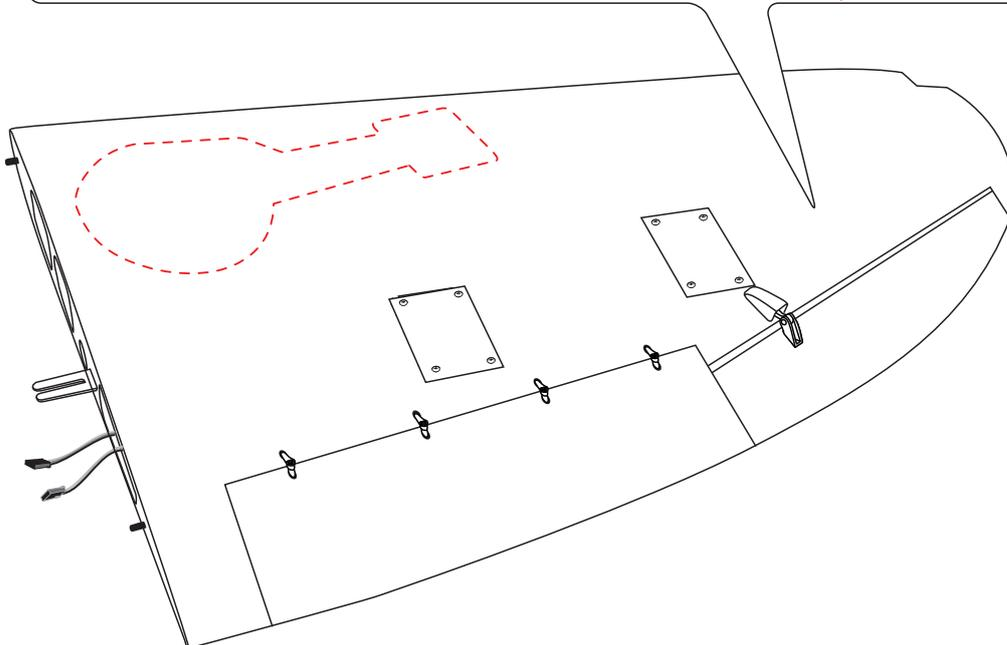
**INSTALLING GUN AND LIGHT PART FOR WINGS**
