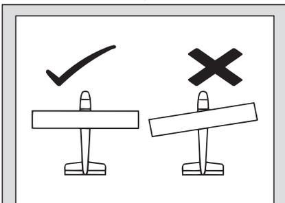
Check that the wings are correctly fitted to the fuselage.
