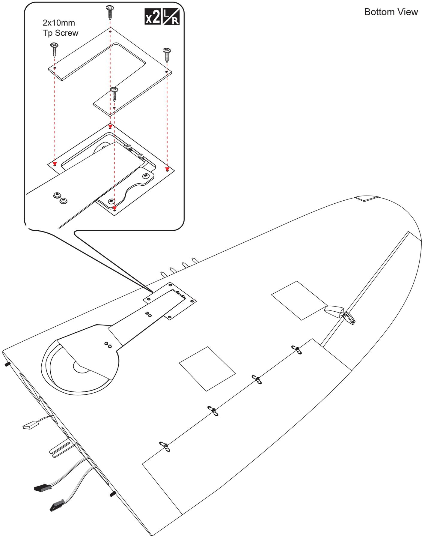
**INSTALLING BOMB PART FOR WINGS**
