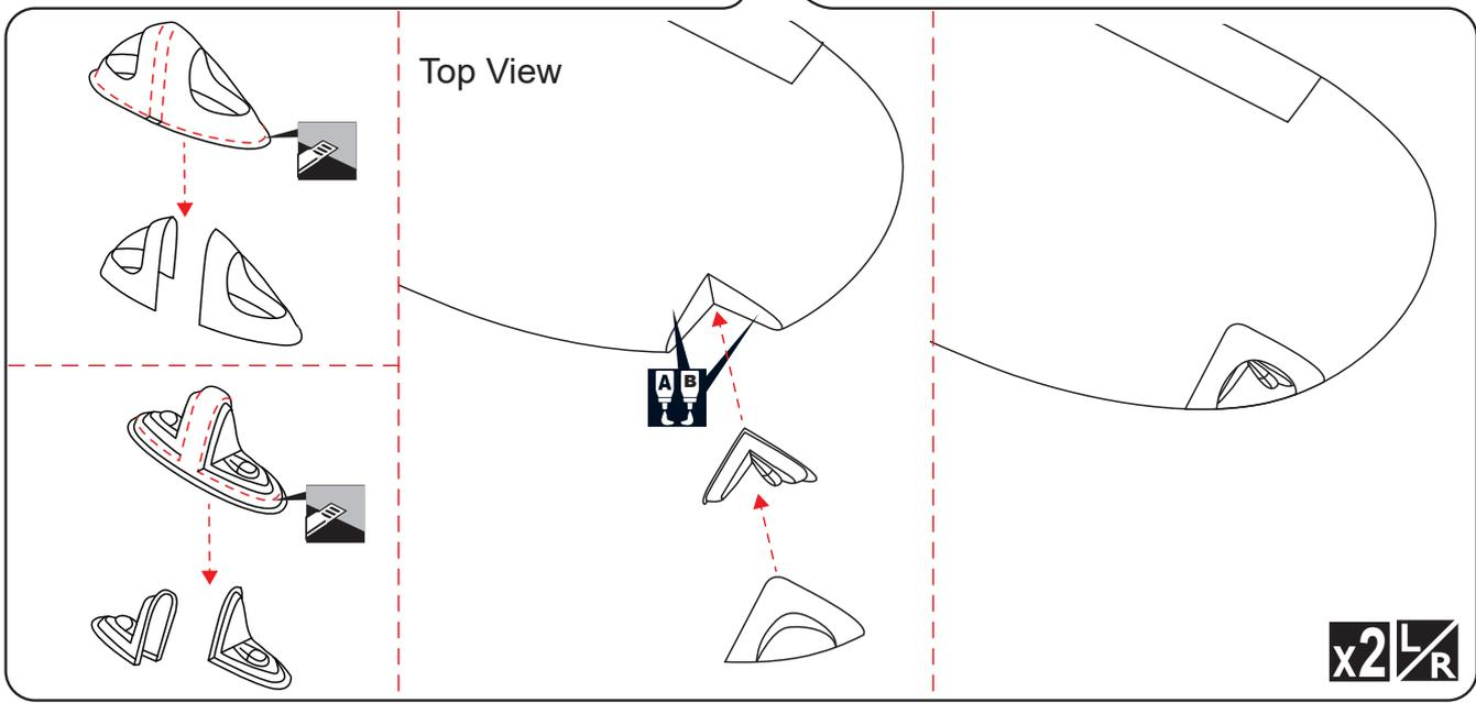
**INSTALLING THE ELECTRIC RETRACTABLE LANDING**
