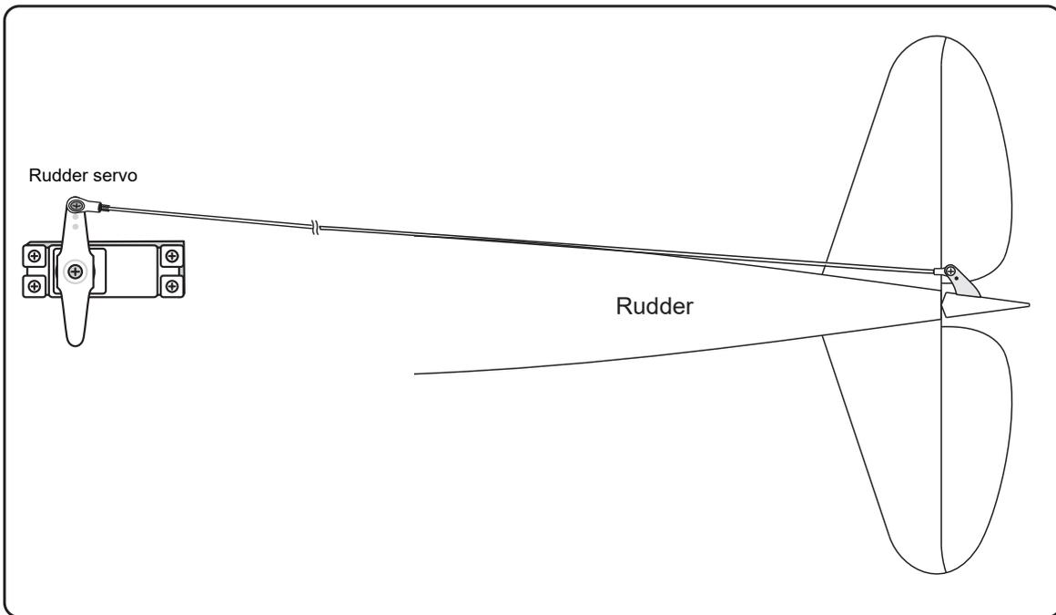
**INSTALLING THE TAIL GEAR**
