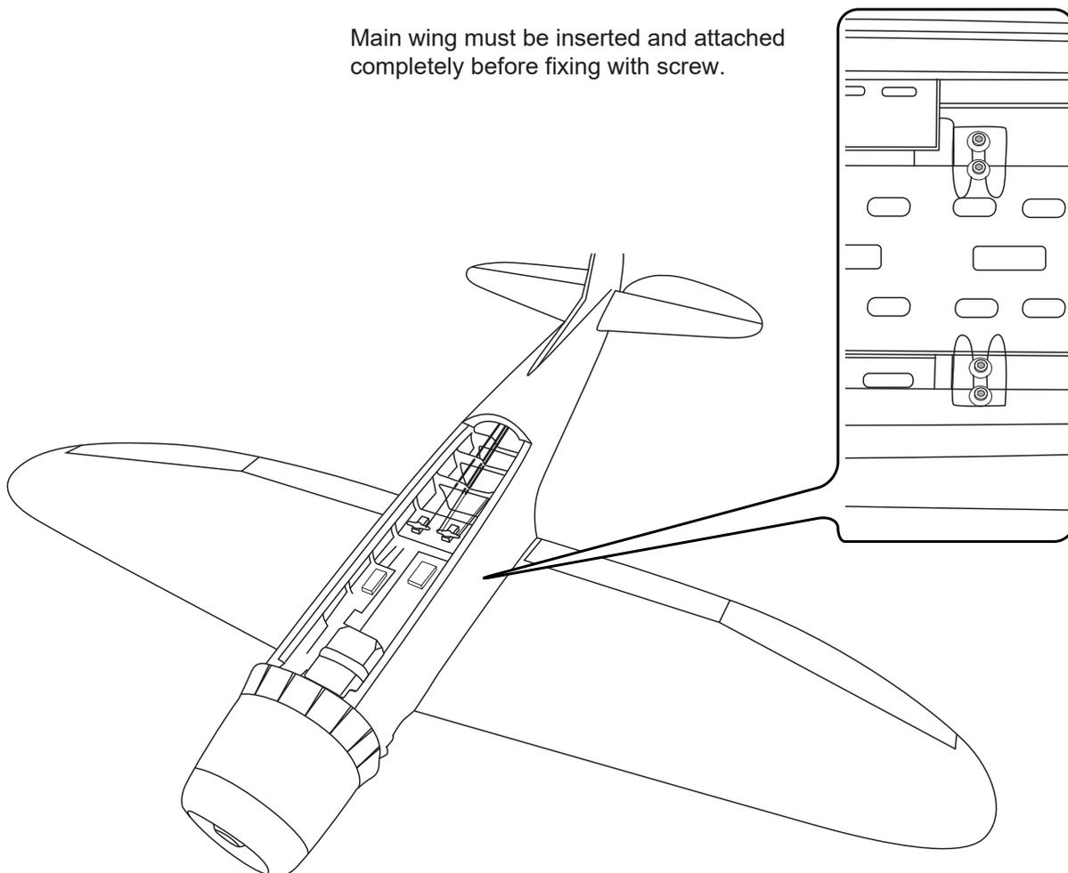
**INSTALLING COCKPIT FUSELAGE**
