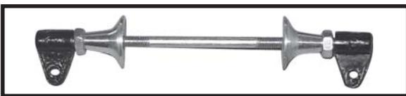
Control horn of Rudder.
