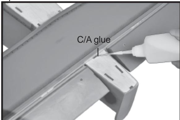
□ 6. After the epoxy has fully cured, remove the masking tape or T-pins used to hold the stabilizer in place and carefully inspect the glue joints. Use more epoxy to fill in any gaps that were not filled previously and clean up the excess using a paper towel and rubbing alcohol.
