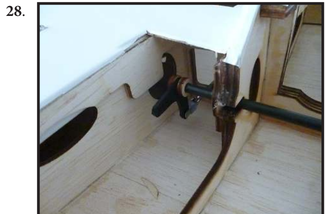
Finished gear door servo/control rod.
