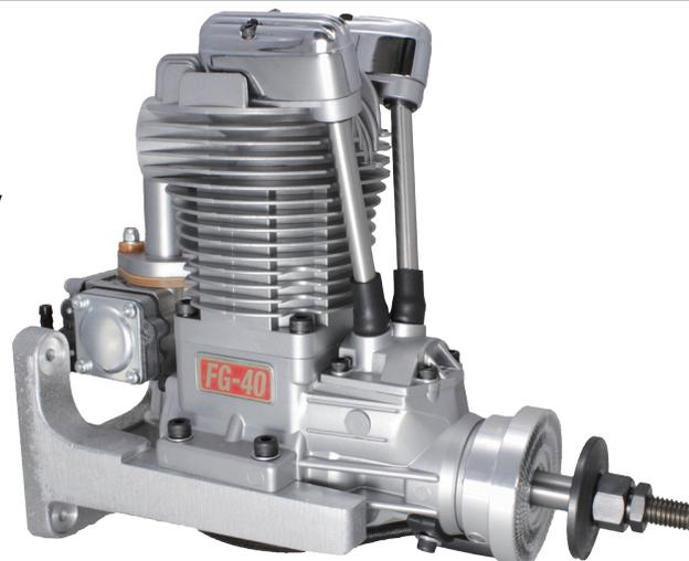
FG-40 has stronger torque by virtue of bore up based on existing gas-engine FG-36. New ignition system brings stability and easy handling. Since its outer dimension including the mount is just the same as FG-36B (the new ignition model of FG-36), it's easy to replace FG-40 with 36B.
