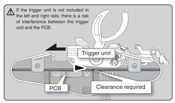
Look inside from the removed rear unit side and insert the trigger unit while checking the clearance between the PCB and the trigger unit. Be careful as the PCB and the trigger unit will be damaged if they interfere with each other.
