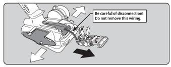
Remove the trigger unit, there is a window at the spring. First, loosen the trigger spring tension to the maximum, remove the spring from the window with tweezers, etc., and replace it.
