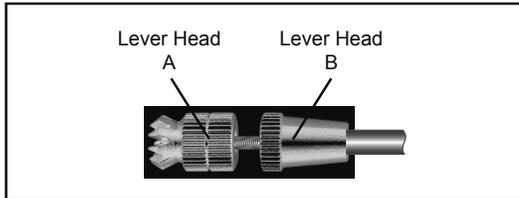
1. Hold the lever head "B" and turn the lever head "A" counter-clockwise, the lock will be released.
