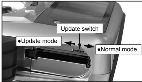
1. Insert the CF card containing the update file into the card slot.
