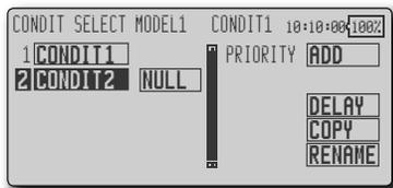
3. Move the cursor to [NULL], call the switch setup screen by pushing the enter button, and select the switch and ON direction to be used in condition switching.
