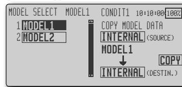
4. Use the cursor lever to move the cursor to the copy source model in the model list and then push the enter key.
