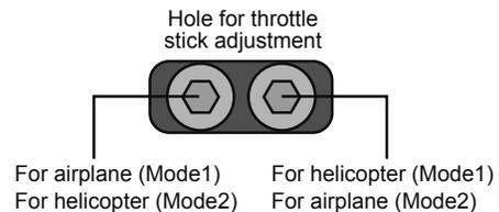
\*This transmitter has two ratchet plates, one for airplane and the other one for helicopter. If you tighten both screws, you won't be able to achieve the adjustment that you need because of the overlap of those two adjustments.
