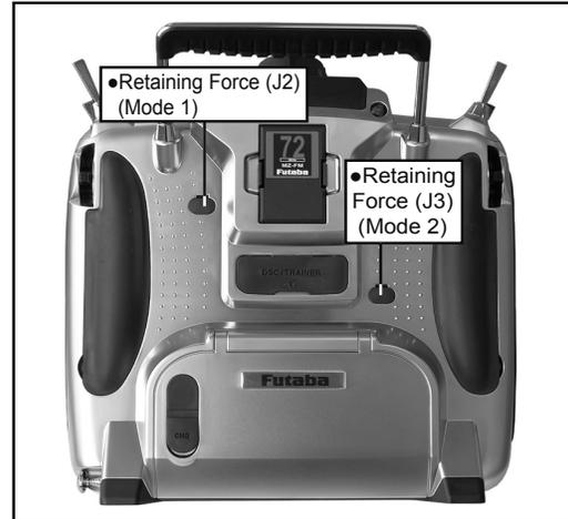
1. Open the dust protection cap on the back of the transmitter that is covering the hole for throttle stick adjustment.
