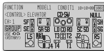
2. Use the cursor lever to move the cursor (blinking) to the icon of the control you want to change, and push the enter button.
