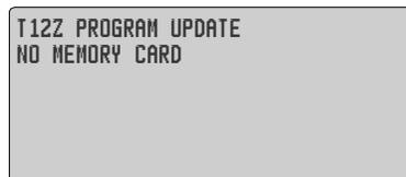
4. When the enter button is pushed about 3 seconds, updating starts. During writing, the bar graph moves to the right.
