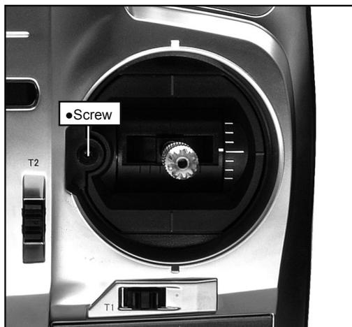
Use the attached 1.5mm hexagonal wrench to turn the screw clockwise to adjust the stick outwards, or counter-clockwise to tilt it inward.
