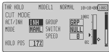
Note: At initial setting, the setting mode is the group mode. Since this function is not used at other conditions, switch to the single mode before setting.
