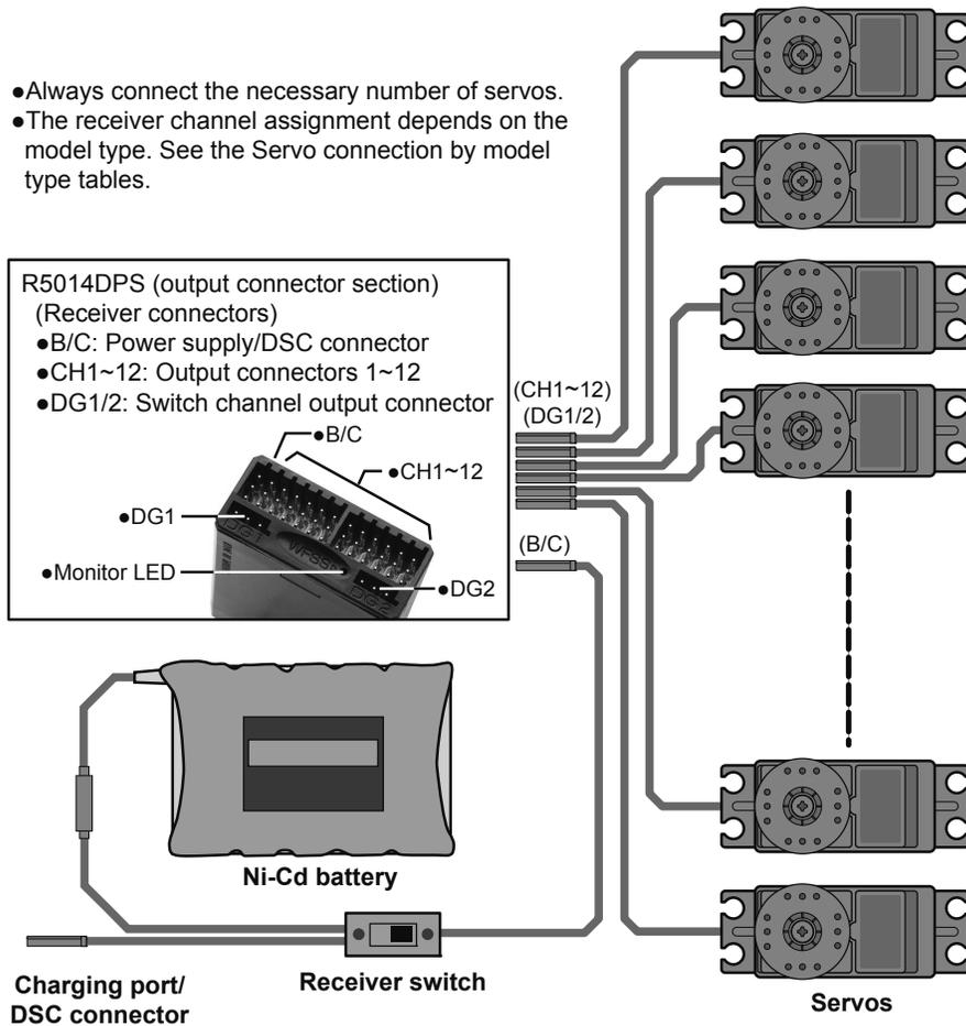
The Servo connection by model type tables are shown on the following pages. Connect the servos to match the fuselage used.
