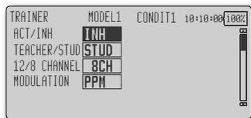
Note: In "student mode", only the teacher side can turn on and off the power to the student's transmitter. Keep the power switch always at off position. Note: In "teacher
