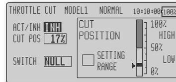
\*With throttle stick at idle, adjust the cut position until the engine consistently shuts off, but throttle linkage is not binding. When finished, push the return key to exit.
