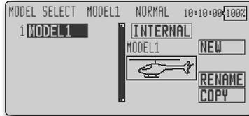
This is convenient when calling a model after registering the model names in advance. (The data of up to 25 models can be saved at the transmitter. Data can also be saved to the optional CF card.)
