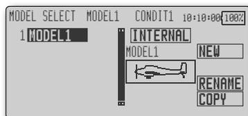
The data for up to 25 models can be saved to the transmitter. Data can also be saved to the optional CF card.
