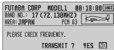
2. Check the frequency shown on the screen. If it is OK, then select [YES] and push the enter button.
