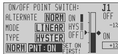
2. When you want to change the mode or type, move the cursor to [MODE] or [TYPE] and switch the display to the mode or type you want to change by turning the data input dial to the left or right and then make the change by pushing the enter button.
