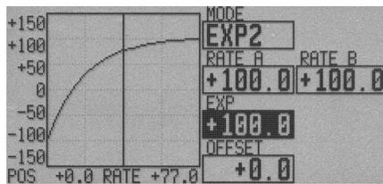
Using the EXP2 curve is effective in engine rise and other engine control.
