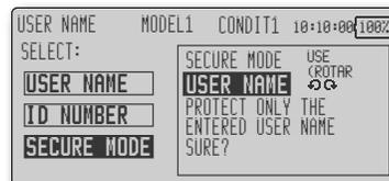
1. When confirming and changing the security mode in the box at the right side of the screen, turn the data input dial. The display starts to blink. When the enter button is pushed, the display lights steadily and the mode actually changes.
