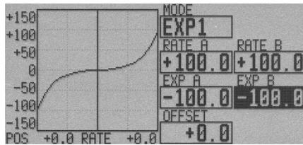
Using the EXP1 curve is effective in smoothing starting of the ailerons, elevator, rudder, etc.
