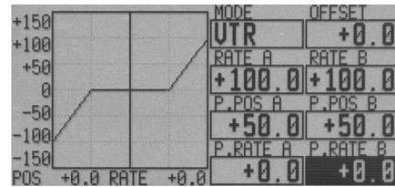
When this curve is used, when the operating rudder angle is large such as with acrobatic models, switching from normal flight to acrobatic rudder angle is performed without switch operation.
