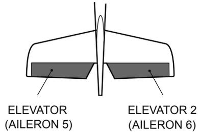
Note: Select Ailevator as the Model Type at the Model Type screen. This changes the output channel. Check the Function menu.
