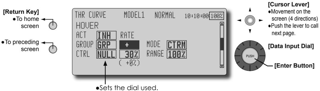
The Throttle Hover function trims the throttle near the hovering point. Normally, use it with hovering conditions. Changes in rotor speed accompanying changes in the temperature, humidity, and other flight conditions can be trimmed. Adjust the throttle so that rotor rotation is most stable. More delicate trimming is also possible by using this function along with the Hover Pitch function.
