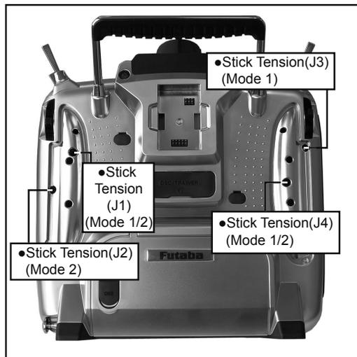
2. Use the accessory 1.5mm hexagonal wrench to adjust the spring strength as you prefer by turning the adjusting screw of the stick you want to adjust.
