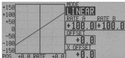
The curve left and right rates ([RATE A], [RATE B]) can be adjusted separately.
