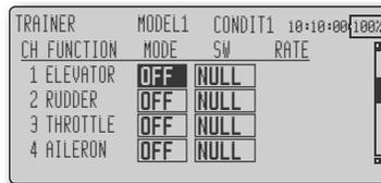
\*Use the cursor lever to move the cursor to the "MODE" item of the channel you want to change and change the mode by turning the data input dial to the left or right. The display blinks. Press the enter button to change the mode.
