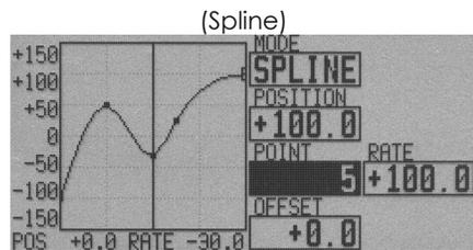
Lines or splines of up to 17 points can be used. (Initial value: 9 points) The set points can be freely increased, decreased, and offset.
