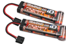
Two 7-cell NiMH battery packs with Traxxas High-Current Connectors*
