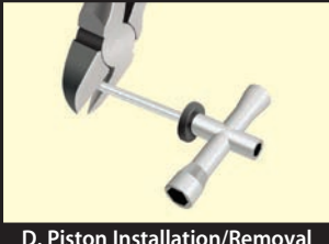
D. Piston Installation/Removal
