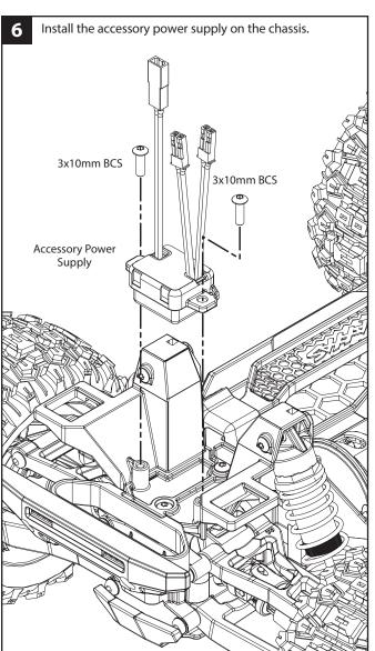
**Important Note!** Use the included power tap as the direct battery source for the accessory power supply. Do not connect to the accessory BEC power output on the ESC (if equipped). Connecting high-load accessories to the power supply while it is plugged directly into the ESC could overload the speed control's BEC circuit. This may cause the speed control to go into thermal protection mode or could cause damage to the speed control.
