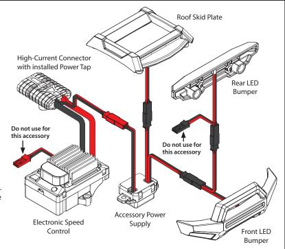
Plug the red male connector from the power tap into the red female connector from the accessory power supply. The accessory power supply and LED lights will turn on when a battery is connected. Always disconnect the battery when not in use.
